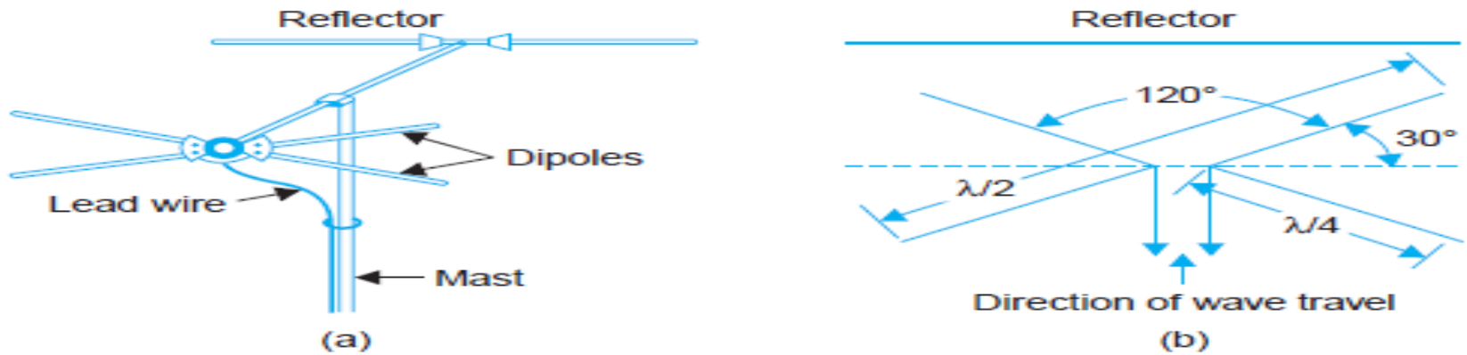
Fig. 9.21. VHF fan (conical) dipole with reflector (a) pictorial view, (b) spacing of elements.
