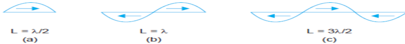
Fig. 9.7. Current distribution on resonant dipoles.
